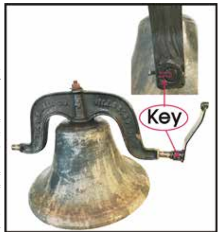
This diagram shows where I had to machine the bell so the lever would grab the shaft.
